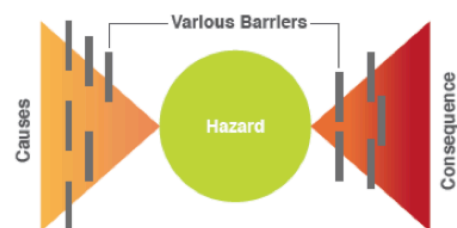
A "bow tie" diagram enables us to identify risks and the barriers to prevent a hazard escalating into a major accident
